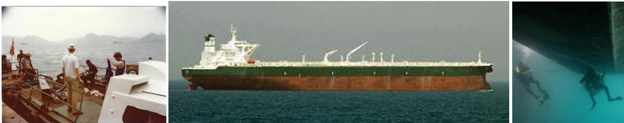
Figure 8/9/10: Scuba diving under VLCC for coating inspection, Sources: Charles. B Harvilcz, Wikipedia, Defense.gov
