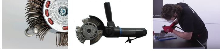
Figure 11: Cleaning metal surfaces with motorized patented device with metallic brushed wires
