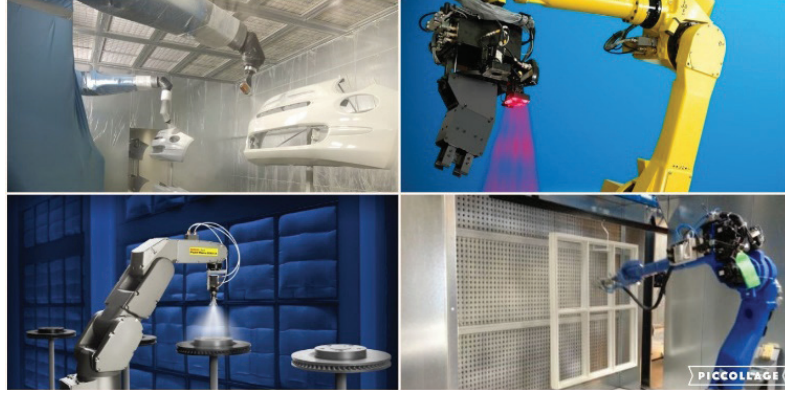
Figure16: Auto-matic Painting with Robotic Systems
