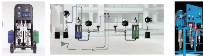
Figure 13: Multi-component Paint Spraying Application with Electronic Proportioner Systems.
