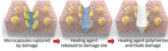
Figure 4: Micro-encapsulation-based Self-Healing/Self-Repair Paints and Coatings and the simple operation mechanism
