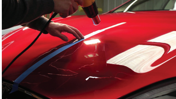
Figure 5: Self-healing / repairing of the paint by applying heat to the scratched paint on the vehicle
